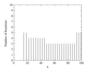
Fig. 6. Number of iterations needed for finding the zeros of  $J_{10}(x)$  in the interval [1, 100].
